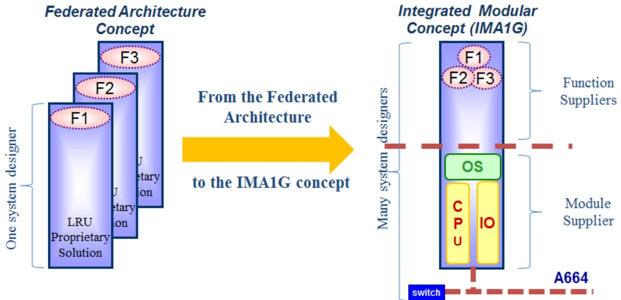
Fig. 1 The Federated Architecture concept vs. the IMA1G concept
