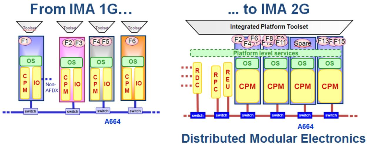
*Fig. 2 Innovation beyond IMA1G – Distributed Modular Electronics*
