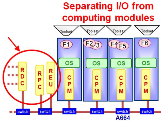
Fig. 3 Separating I/O from computing modules
