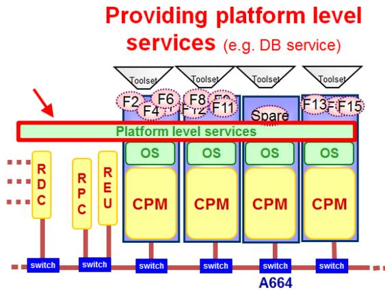
Fig. 5 Providing platform-level services
